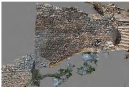
Fig. 8- Combination of photos with different lighting – dense point cloud.
