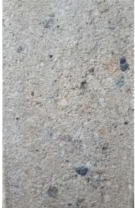
Fig. 3- Conglomeratic sandstone lithofacies the Montjuïc Sandstone. In most the rock is matrix supported with the clast, mostly silicic (rounded vein-type white clasts, coming from the palaeozoic substrate now outcropping at Collserolla hill; and blackish rounded fragments of chert, Silurian of Carboniferous in age). From time to time the clast-bed show higher porosity that the usual Montjuïc sandstone lithofacies (private apartment, Carrer Josep Anselm, Barcelona).
