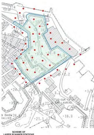
Fig. 4- Birgu, Malta. Scheme position of laser scanner.
