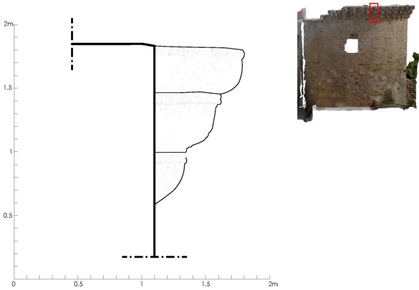
Fig. 10- Detail of the corbels, side elevation (Griffo, 2018)
