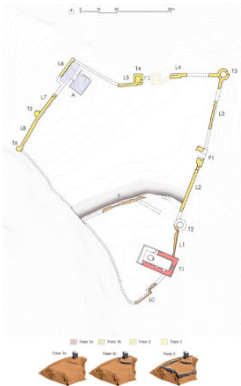
Fig. 3- Plan and hypothesis of the main phases of construction of the Castle of La Peña (graphic elaborations by the authors)
