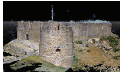
Fig. 6- Castle of Torres Vedras, circular tower that housed the artillery, view of the dense point cloud, obtained through the process of aerial photogrammetry and identification of the acquisition points (Fabiana Guerriero, 2021).
