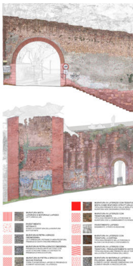
Fig. 11- Architectural two-dimensional vector representations of the subdivision of portions by type of masonry found
