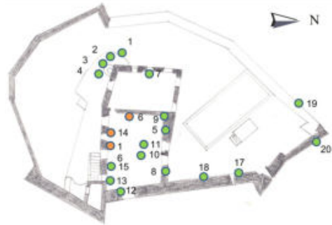
Fig. 7- Localization of samples (orange = bricks; green = mortars) (graphic elaboration by Silvia Rescic)
