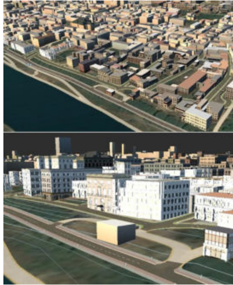
Fig. 6- Mesh model of the city of Pavia visible within the Autodesk Infraworks viewport. On the bottom, the details of the area near Porta Nuova. The monument of the gate is not reliable in its complexity, but it is greatly simplified, highlighting how the basic model from available territorial maps needs to be supplemented with additional architectural and urban details (Francesca Galasso, 2021)
