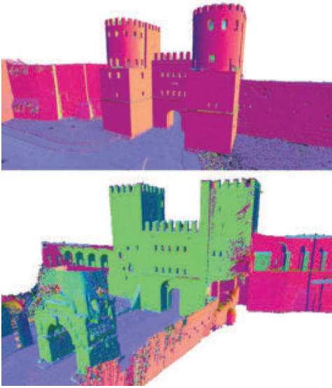
Fig. 1 - Integrated point cloud of the Gate and the Arch (graphic elaboration by authors)
