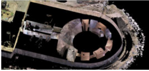
Fig. 7- Entrance, access ramp and laser scanner survey of the Fort Campana (graphic elaboration by A. Altadonna)
