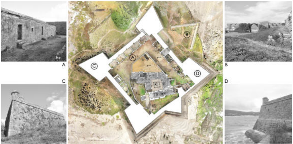
Fig. 2- Spatial organisation and defensive system components of the Fort of Ínsua. Military lodging (A), external tenaille (B), western bastion (C), eastern half-bastion (D) (graphic elaboration by Rolando Volzone, 2022)
