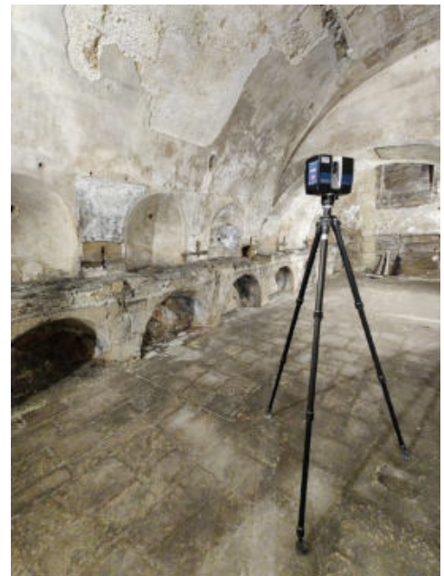
Fig. 4- The 3D laser scanner unit in front of the Putridarium beneath Palazzo Stola (Giorgio Verdiani, 2021)
